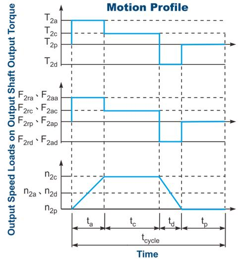
$$1. ED = \frac{t_a + t_c + t_d}{t_{cycle}} \times 100\%, t_{work} = t_a + t_c + t_d$$
