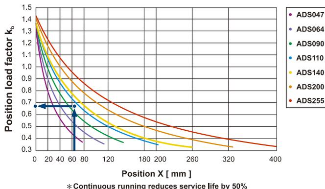
If radial force  $F_{1r}$  is exert on the center of the output shaft  $X=1/2 \times L$ . The permitted radial load is given on above diagram.
