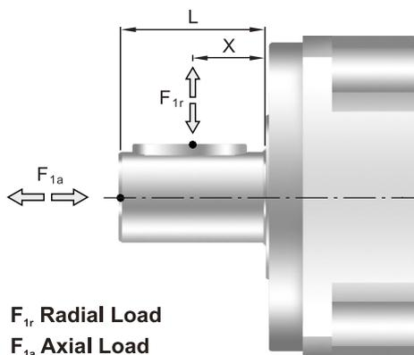
The permitted radial and axial loads on input shaft of the gearbox depend on the design of the gearbox supporting bearings. APEX use the extension straddle oversized ball bearing design. It can take heavy load from both axes.
