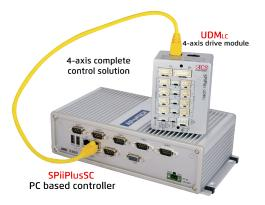
The unit is powered by a 12 to 48Vdc drive supply voltage and by a separate 15 to 48Vdc control supply that keeps all logic signals alive during emergency conditions. The UDMLc is panel or din rail mountable.
