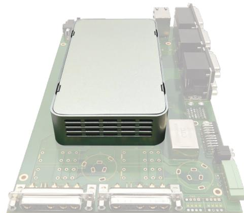
The UDM<sub>CB</sub> is a line of economical and compact PCB mounted EtherCAT drive modules.
