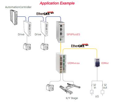
The SPiiPlusES is a high performance programmable motion controller and EtherCAT Master that can be connected as a node to any EtherCAT network utilizing the standard DS402 CAN Over EtherCAT (CoE) protocol. To the external EtherCAT Master it looks like a highly programmable multi-Axis motor drive.
