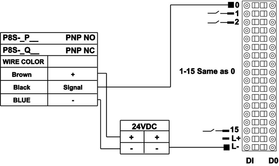
The above connections apply to both the P8S and P8S Mini-Global Sensors, shown on the next two pages.
