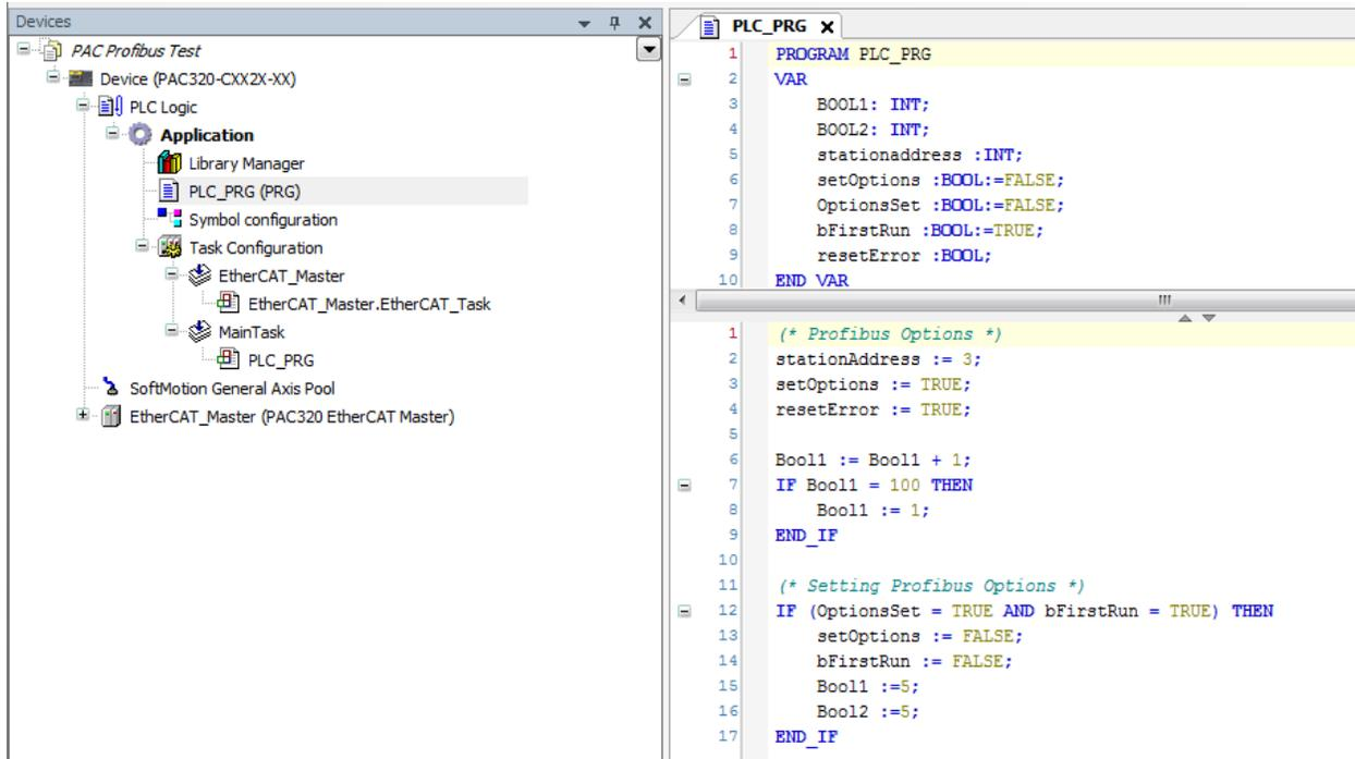
2. After adding the device and code to the project, you will configure the IO map as displayed:
