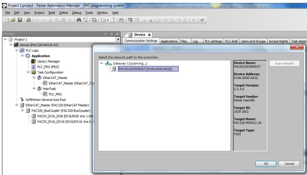
If the scanning process does not find your PAC, double check the subnet mask on the PAC Ethernet port and your computer’s Ethernet port. The subnet mask on both need to match (the default on the PAC is 255.255.0.0). Alternatively, you could just type in the IP Address of the PAC in the right side drop down box on the Communications Setup tab from the previous step.
