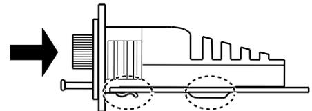
7. To lock the Module into the Controller, push the handle of the sliding latch fully into the Module.
