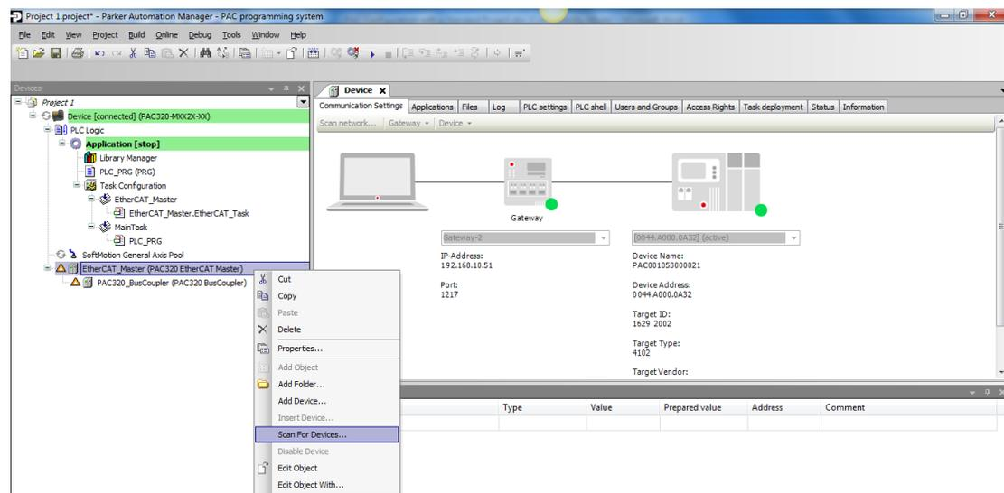
3. A list of connected EtherCAT slaves will be displayed. If this list is missing a slave, ensure the slave is connected and powered on, and then click the **Scan for Devices** button to re-scan.
