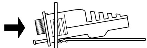
6. Push the Module further into the Controller until the final position is reached and the module cannot be further inserted.
