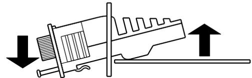
5. Push the module further into the unit until it engages into the internal board cutouts.
