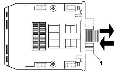
3. Insert the module approximately half way into the cutout opening on the face of the Controller.
