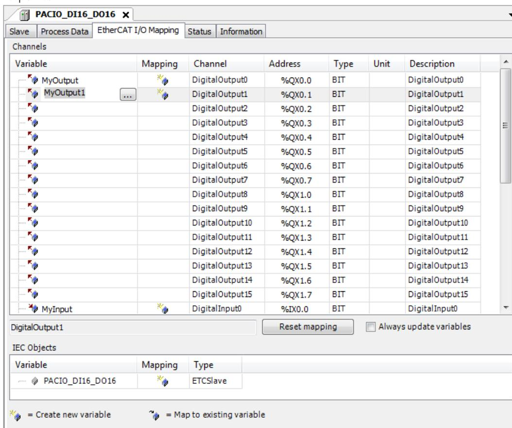
3. Double click in the Variable column for the desired IO point and create a name for this point.
