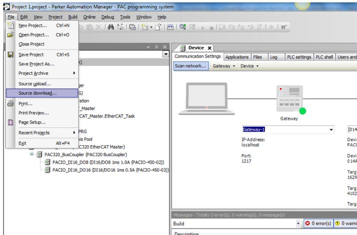
2. Select **PAC320** under the Gateway as the device to download the project. If the PAC does not show up under the Gateway, select **Scan Network** to locate the PAC. Select **OK** to download the project.
