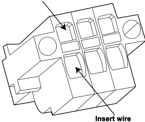
*Attach Wires to Tension Clamp Terminals*
