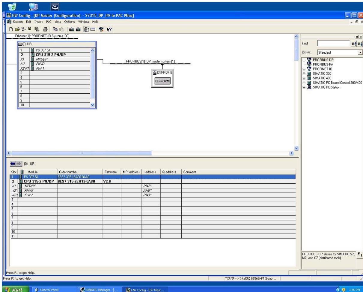
6. Select the X1 Port. Configure the X1 port to Address 2.
