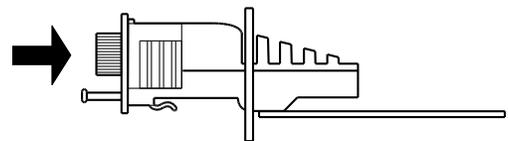
4. Tilt the module slightly downwards and push it further into the Controller.
