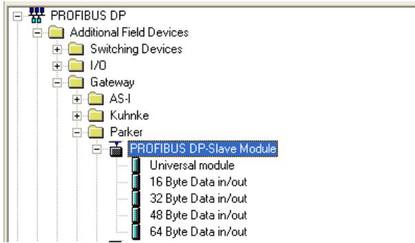
10. Right click on the ProfiBus network and insert the loaded GSD file.
