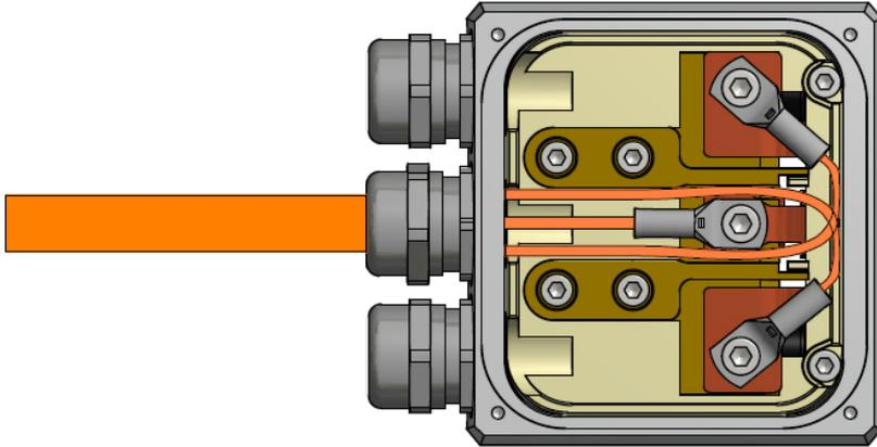
As previously, Parker can provide 4 meter length power cable to take place between the drive and the battery (with 2 interlock wires) which part number is HVLP-B-D-CABLE.
