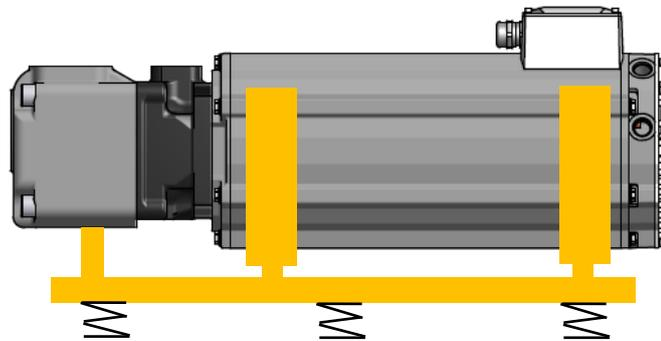
GVM motors have been designed for an horizontal mounting (see §4.2). Considering the above schematics, GVM motors have to be supported on their rear side.
