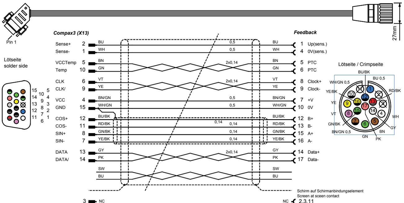
GBK56/...: (cable chain compatible) for EnDat2.2 (cable plan on request)
