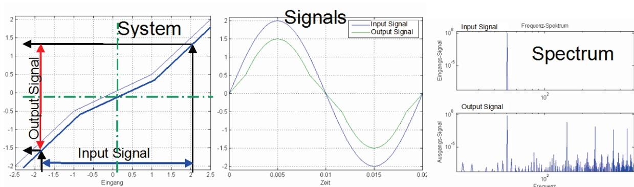
Due to the non-linear transmission behavior of the system, many "new" frequencies were generated in the output signal. In the frequency response, only one change of the frequency present in the input signal can be displayed meaningfully.
