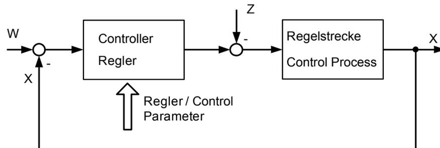
The basic task of a control is the generation and maintaining of a desired state or sequence in spite of interfering disturbances. It is essential that the effects of the disturbances are balanced with the correct force and at the correct time. In the above figure, the setpoint value W represents the desired state and the disturbance value Z represents the interfering disturbance. The actual value X represents the generated and maintained state.
