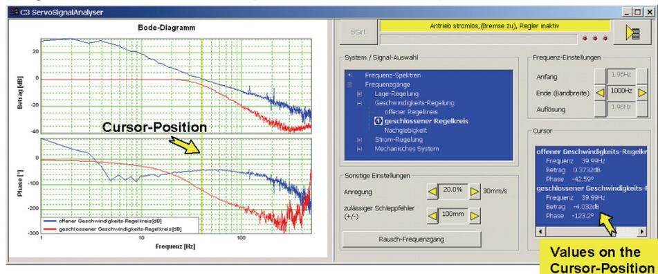
The cursor is set by clicking on the left mouse button. All measurement data of the selected cursor position (frequency) are displayed in the "cursor" operating field.
