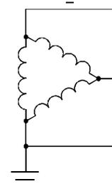
Devices which are to be connected to an IT network must be provided with a separating transformer. Then the devices are operated locally as in a TN network. The secondary sided center of the separating transformer must be grounded and connected to the PE connector of the device.
