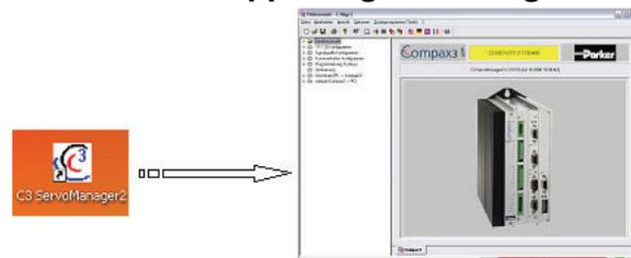
The entry of the motor and application parameters is made with the C3 ServoManager2 (C3Mgr2.exe):
