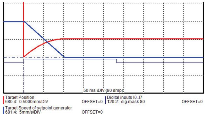
If the homing mode is active, there will always be a homing run with the first start after each configuration download (with the aid of the C3 ServoManager) **Homing run** (see on page 139).
