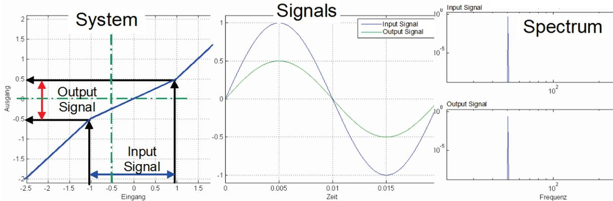
The signal range is reduced so that approximately linear conditions are valid. The results of the measurement will then display the dynamic behavior at the working point.
