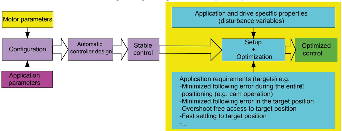
**Overview of the processes during configuration and setup of the Compax3 drive system**
