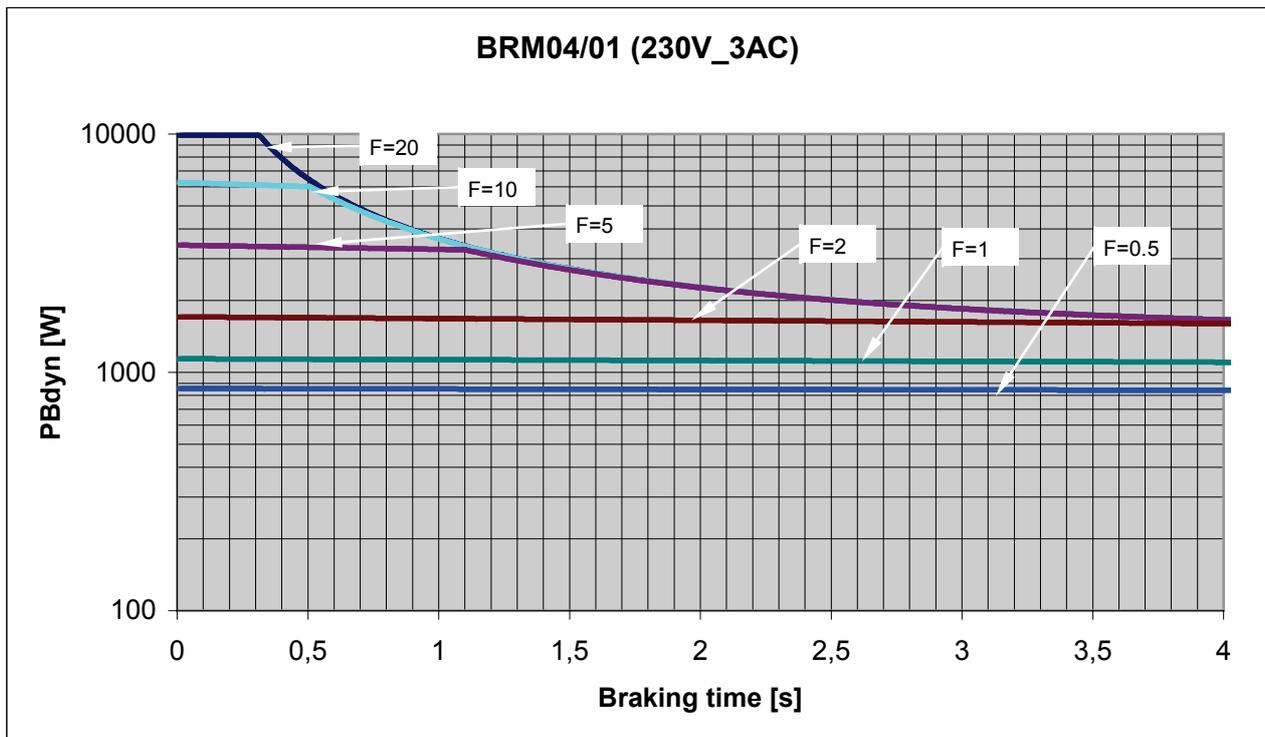
9.4.1.11 Permissible braking pulse power: BRM04/01 with C3S300V4
