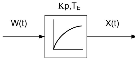
**Step response of a delay component**
