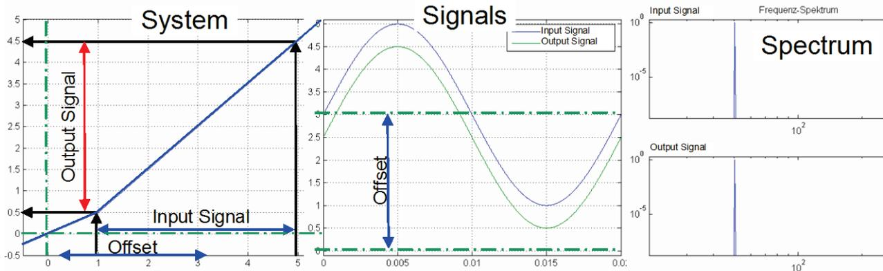
For this, the signal range is shifted so that approximately linear conditions are valid => the results of the measurement show the dynamic behavior at the working point.
