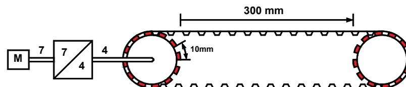
A reset path of 300 mm can be entered directly with numerator = 300 mm and denominator = 1.
