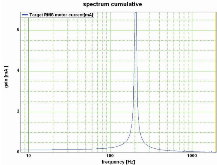
$\Delta f=8\text{Hz} / f_0=204\text{Hz} = 25.5 \cdot \Delta f / \text{frequency}$  does not correspond to the frequency resolution!
