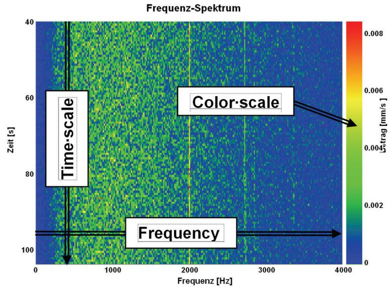
By clicking with the left mouse button on the color scale, you can change between autoscale mode and fixscale mode.
