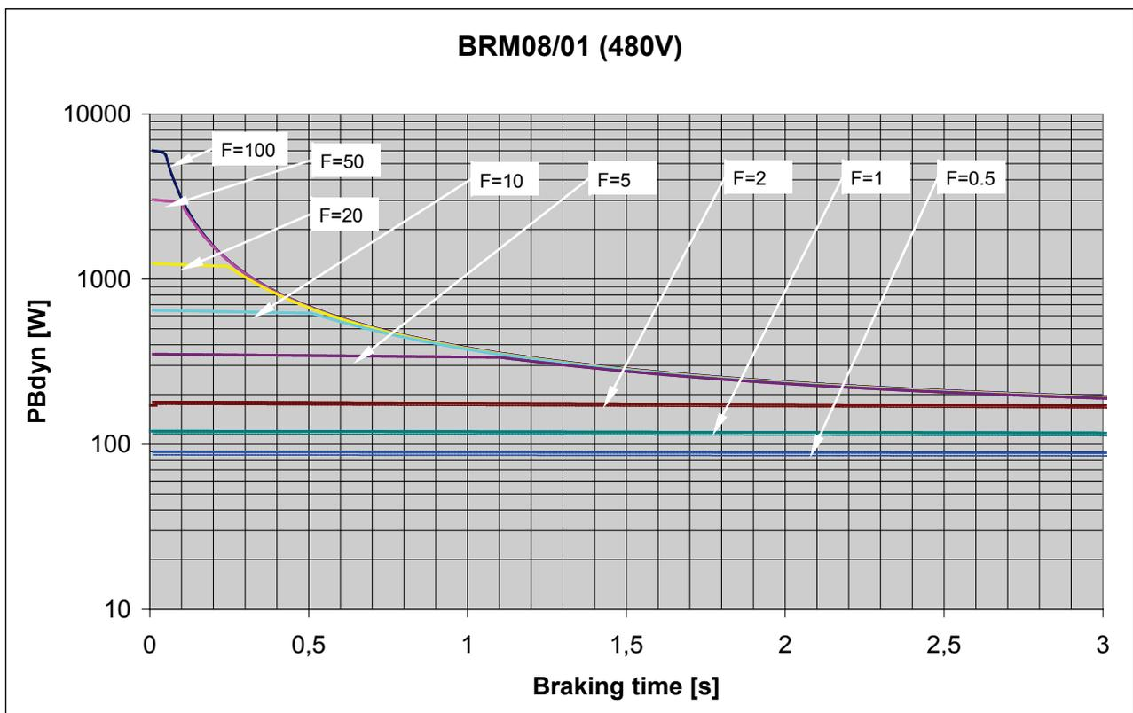
9.4.1.3 Permissible braking pulse power: BRM08/01 with C3S025V2
