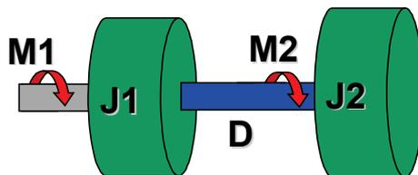
The shown system corresponds for instance to a motor with a flywheel coupled via a shaft. Hereby J1 corresponds to the motor moment of inertia and J2 to the moment of inertia of the flywheel.
