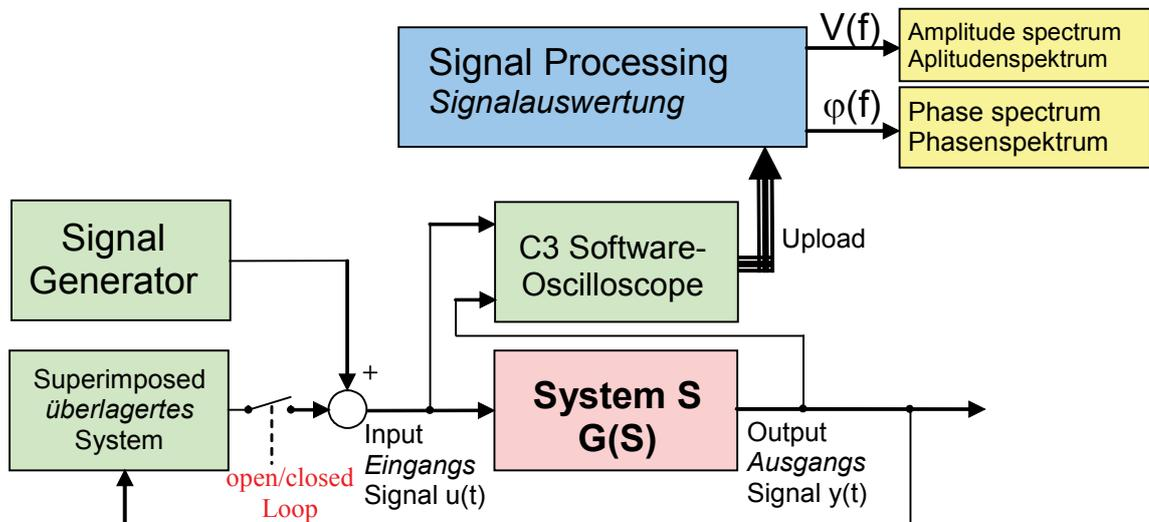
In general, the analysis of the dynamic behavior of a system is made by analyzing the input and output signals.
