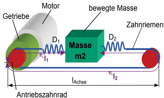
In toothed belt drives, the toothed belt is the elastic coupling element. Its rigidity depends directly on the lengths  $l_1$  and  $l_2$  and changes in dependence of the position of the moved mass.
