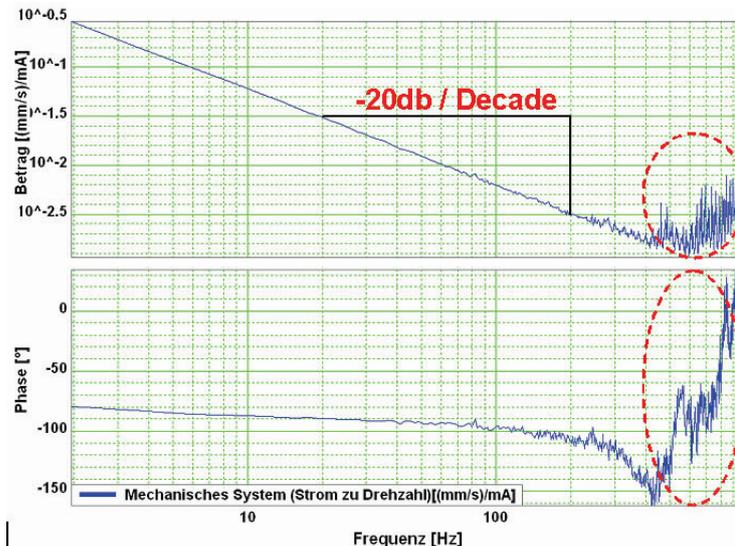
The outlined course at the end of the measurement range does not permit statements on the system measured due to disturbances. Due to the attenuation of the signals increasing with the frequency, the sensitiveness of the measurement to disturbances (signal to noise ratio) increases with a rising frequency. The value as well as the phase response of the displayed frequency response are "disturbed" at the same intensity, this shows, that disturbances are the reason.
