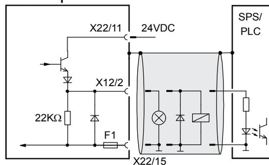
The outputs are short circuit proof; a short circuit generates an error.
