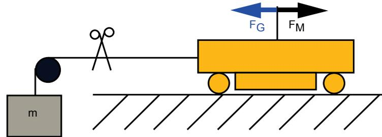
In settled state of the control, the motor force  $F_M$  corresponds exactly to the load force  $F_G = m \times g$ .
