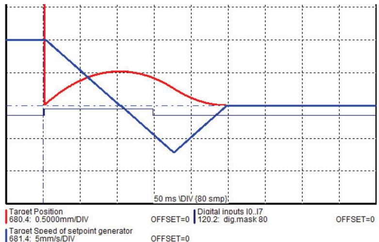
Without positioning after homing run The position reached is not exactly on 0, as the drive brakes when detecting the home and stops:
