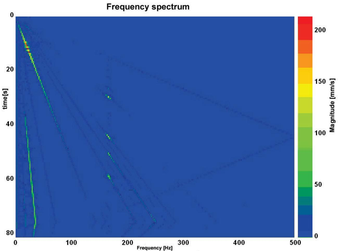
This kind of display is suitable for the analysis of temporal changes in the measured spectrum.
