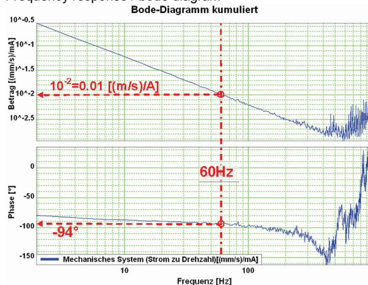
**The frequency response shows the amplification (value) and the phase shift (phase), which a signal is submitted to when passing through a system.**
