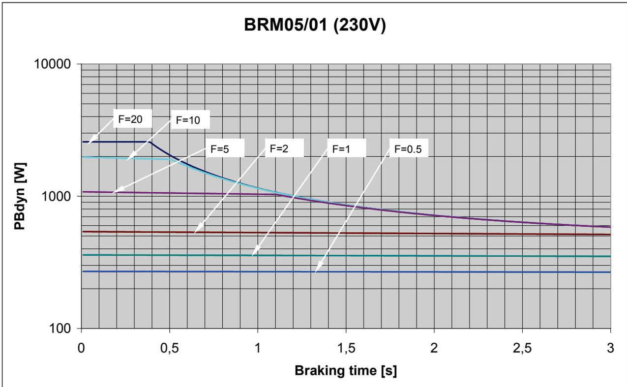
9.4.1.8 Permissible braking pulse power: BRM05/01 with C3S075V4
