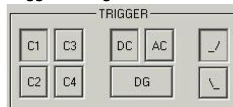
Select trigger channel: Buttons C1, C2, C3, C4
