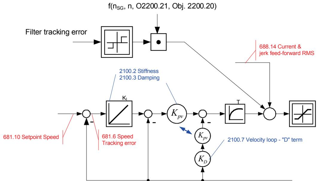
The friction compensation helps the control to surmount static friction at low setpoint speeds. The non linear characteristic line is partly compensated by this and a smaller deadband can be chosen, which will increase the position accuracy. The amplitude of the friction compensation depends on the application and must be calculated if needed. If the value is set too high, corrective movements may result and the tendency to oscillate is increased.
