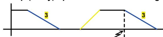
3: Deceleration upon error (malfunction) (ZSW.3 = "1"), OUT1 (CW.0 = "0") and OUT3 (CW.2 = "0")
