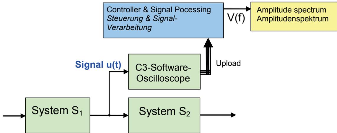
During the spectral analysis of scanned signals with the aid of the discrete Fourier transformation, a so-called frequency resolution ( $\Delta f$ ) results,  $\Delta f$  being  $=fA/N$ , independently of the scanning frequency ( $fA$ ) and of the number of measurement values used ( $N$ ).
