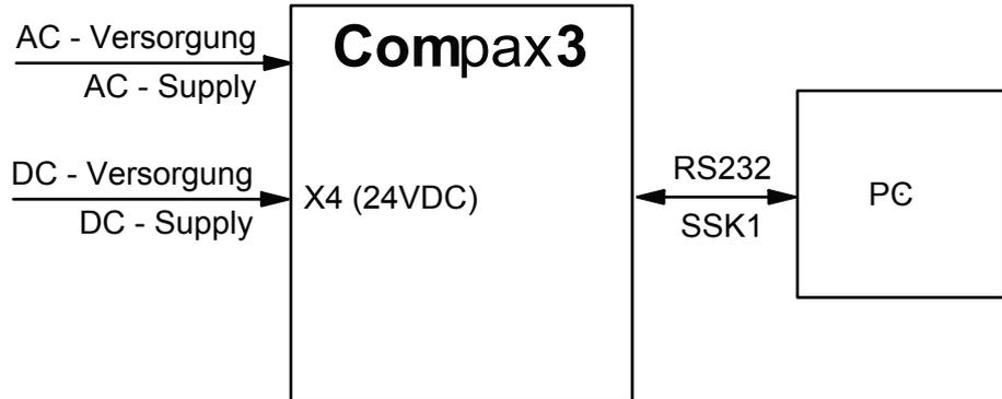
Further information on the assignment of the plug mounted at the particular device can be found below!
