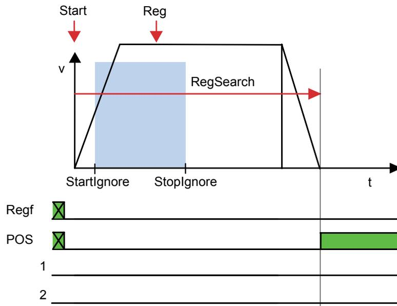
**Start** Start signal for reg positioning (Control word 1 Bit 6)
