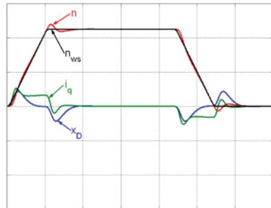
**Velocity, acceleration and current feedforward**
