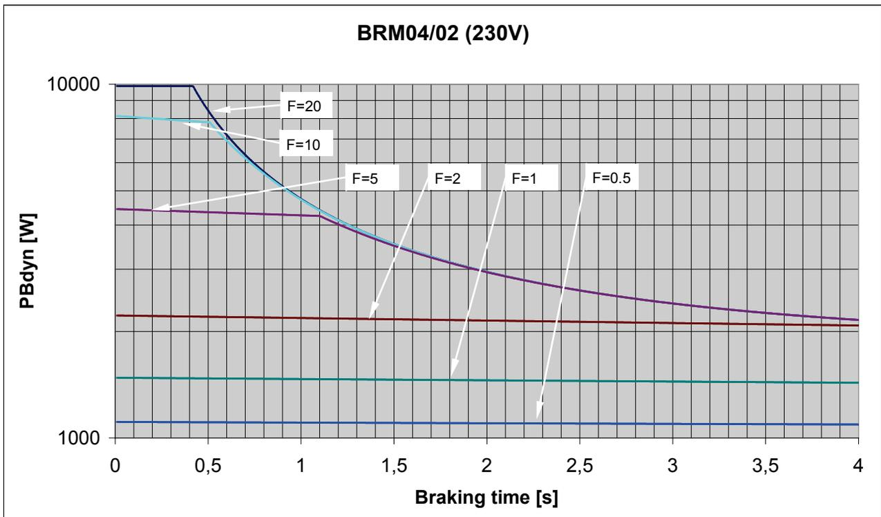
9.4.1.13 Permissible braking pulse power: BRM04/02 with C3S300V4
