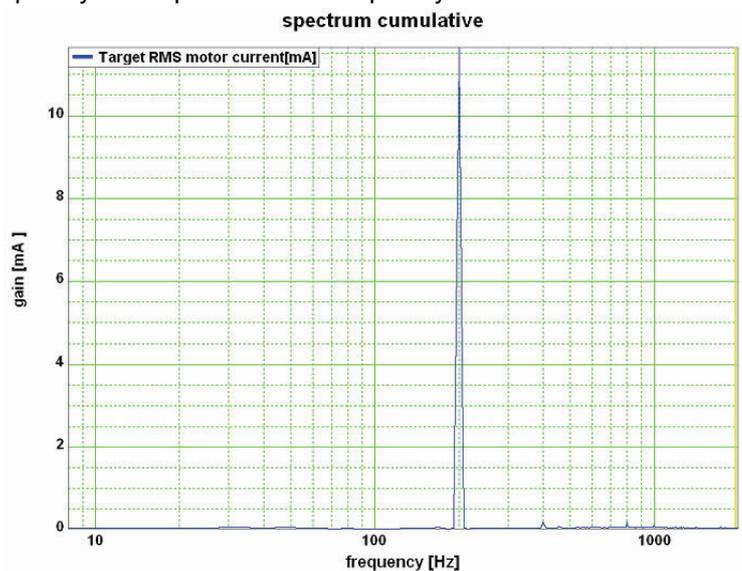
The sine frequency is exactly on a multiple of the frequency resolution (200Hz / 8Hz=25). The spectrum is clearly separated and there are no leak effects visible.
