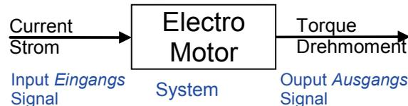
Current is therefore a signal, which causes at the input of the system motor a change of its torque output signal.
