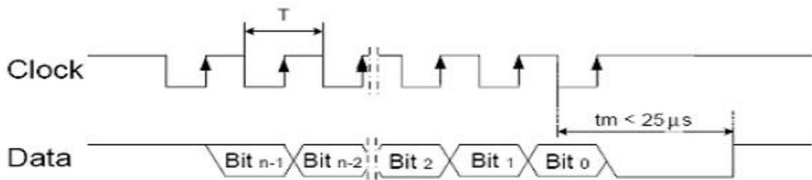
The most significant bit must be transmitted the first!
