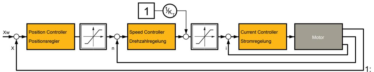
Feeding in of a disturbance current jerk, which corresponds to a disturbance torque jerk.
