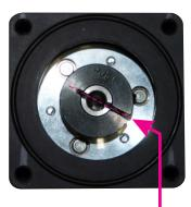
The inner and outer slit is aligned as they should.
