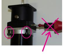
Do **NOT** tighten the shaft collar before the flange bolts are tightend
