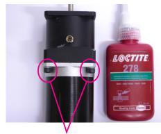
Flange bolts properly mounted and tightend.
