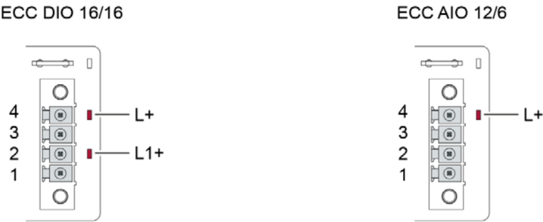
Fig. 4: Power supply at plug X1 with Power LEDs
