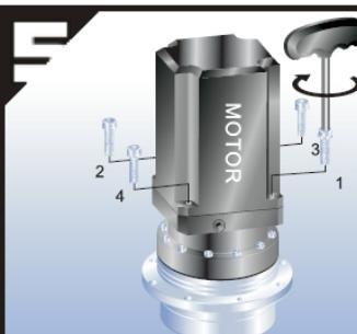
Set at vertical position, tighten the mounting bolts (including washer) in 1~4 order with wrench to 5% specified torque (see table 1)
