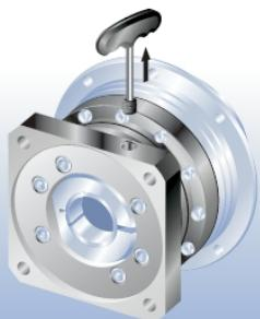
Remove the plug on the adapter plate
