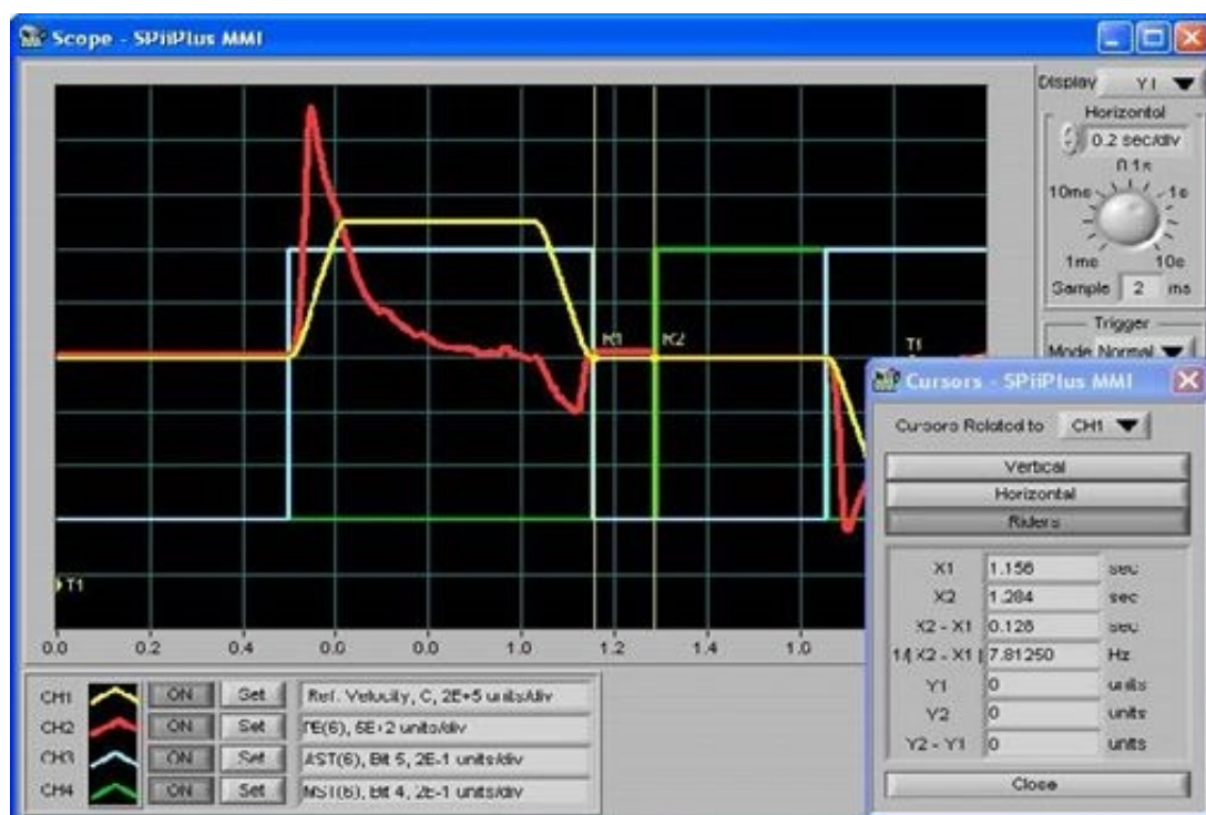
Figure 18-1. Measuring Settling Time (Piezoceramic Motor Example)
