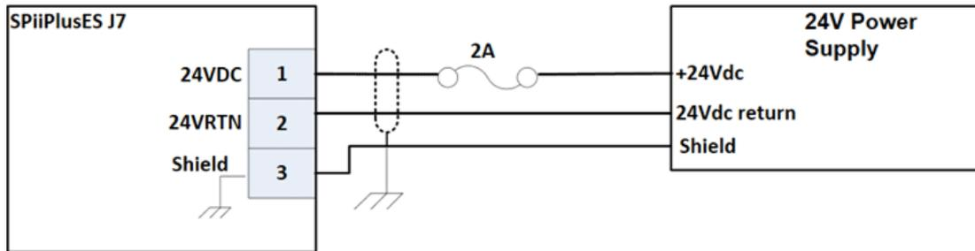
Figure 4-6. Control supply wiring
