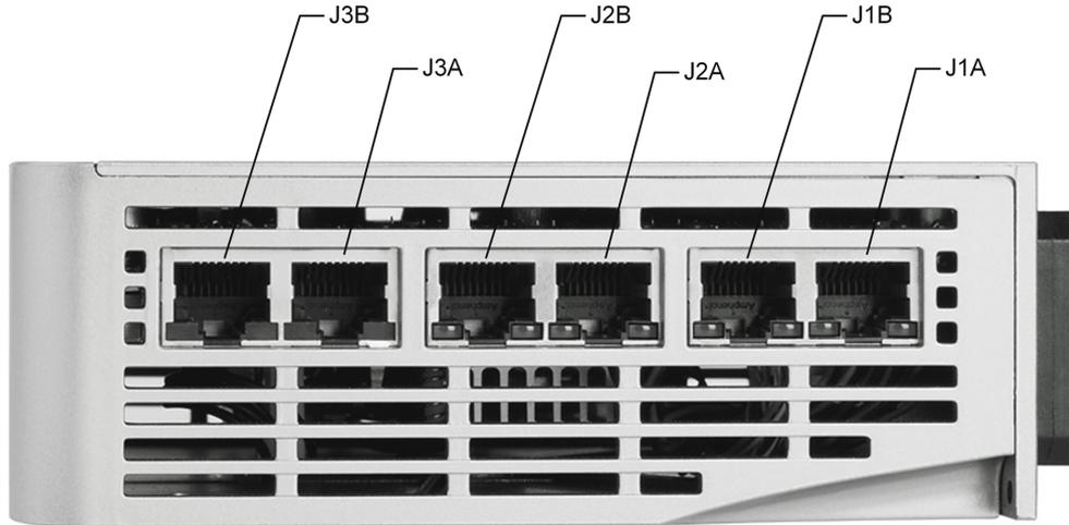
**Figure 2-2. Connectors - top view**
