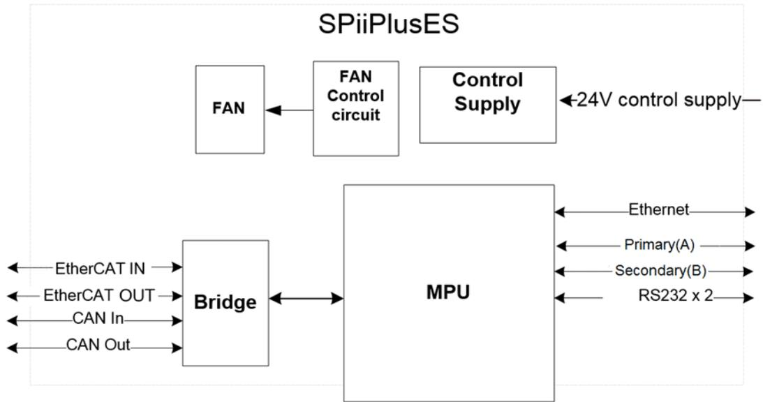
Figure 1-1. IDMSMECMSUDMSM block diagram
