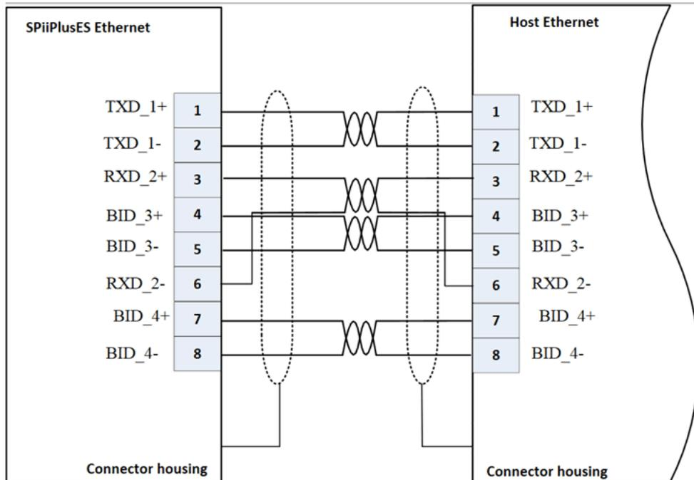
Figure 4-3. Ethernet wiring
