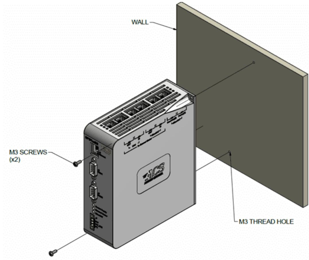
Figure 3-1. Wall installation
