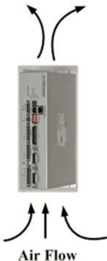
Figure 3-2. Vertical installation with cooling fan
