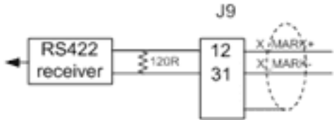
Figure 7-5. Differential Connection for MARK1 Input
