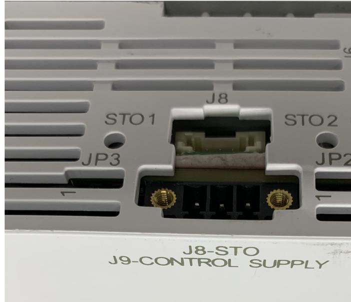
Figure 4-2. J9 - Control Supply Connector
